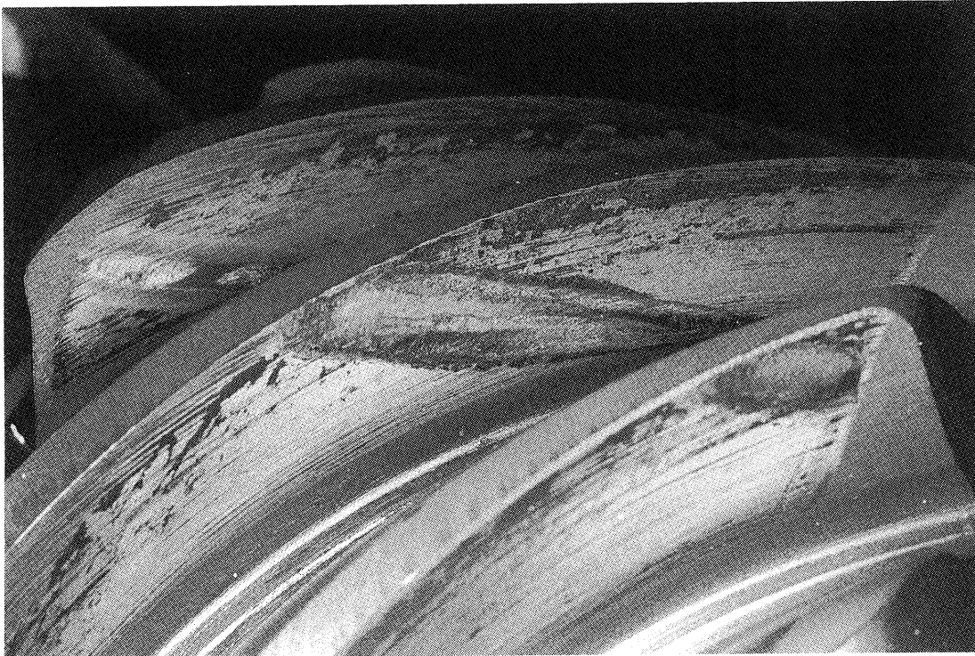
Fig. 2.8 Contact Lines on a Hypoid Pinion
